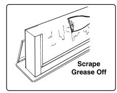
5. Using a nylon or other soft-touch spatula, lift the accumulated grease from the back panel - behind the filters. Clean front and back panels using a mild grease solvent (See Cleaning Chart for Stainless Steel).
